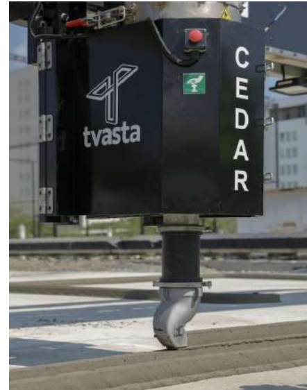
Photos above and right: The Cedar 3D Concrete Printer. Photo credit: Tvasta
